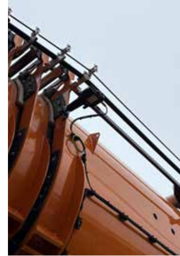
MVRD5200 radio system on a mobile crane
