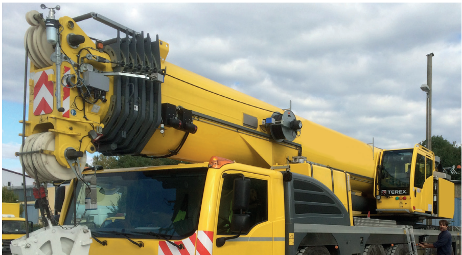
An all-terrain telescopic crane fitted with a Motec camera and monitor system.
