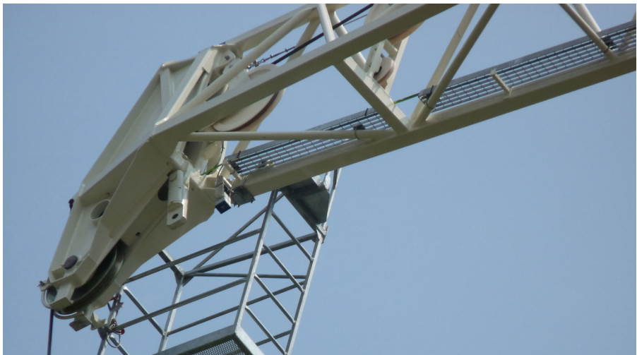
Motor zoom camera at a jib. The pendulum mounting allows the camera to adapt to the jib's tilt angle.
