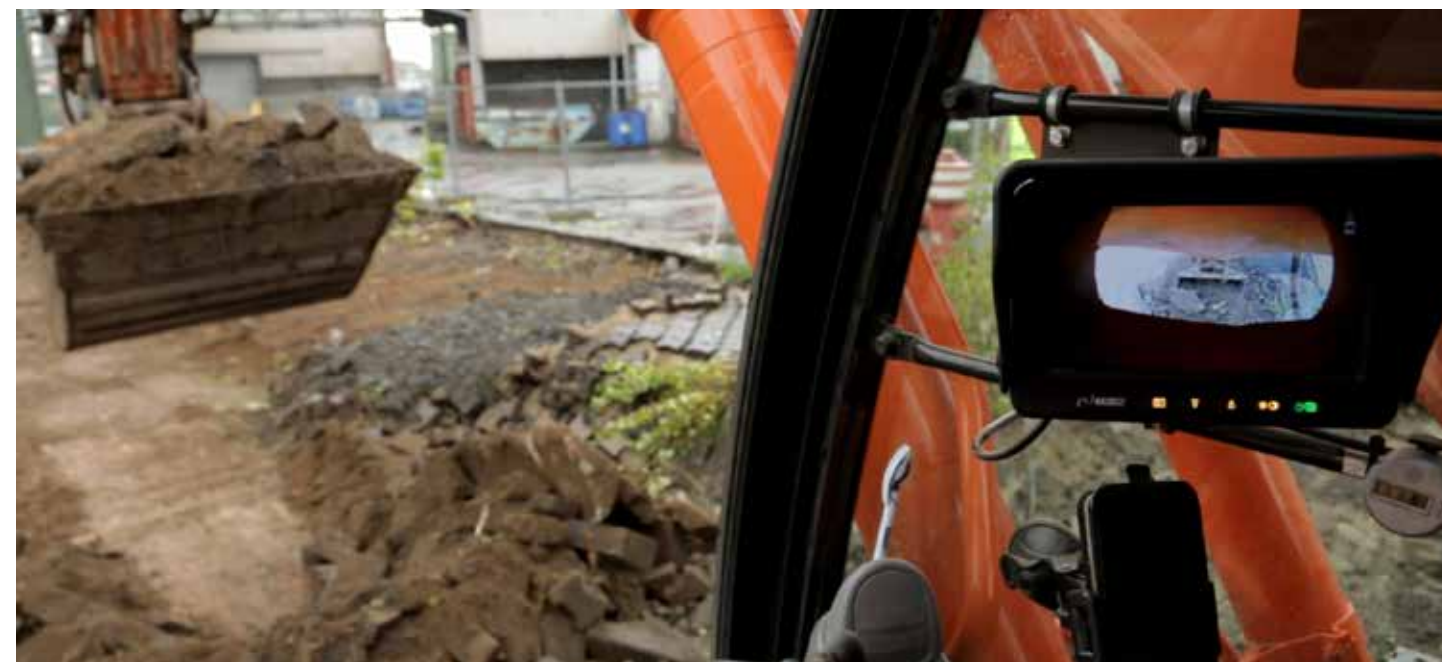
Load monitoring with the MC7180 heavy-duty camera.
