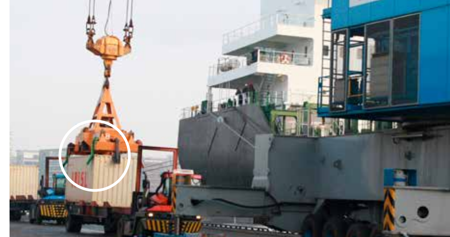
Container bridge with spreader. Twistlock cameras help in centring the spreader during positioning on the container.
